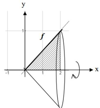
$$V = \pi \int_0^2 \left(\frac{1}{2}x\right)^2 dx = \pi \int_0^2 \left(\frac{1}{4}x^2\right) dx = \pi \left[\frac{1}{12}x^3\right]_0^2 = \frac{2}{3}\pi \cong 2,09$$
